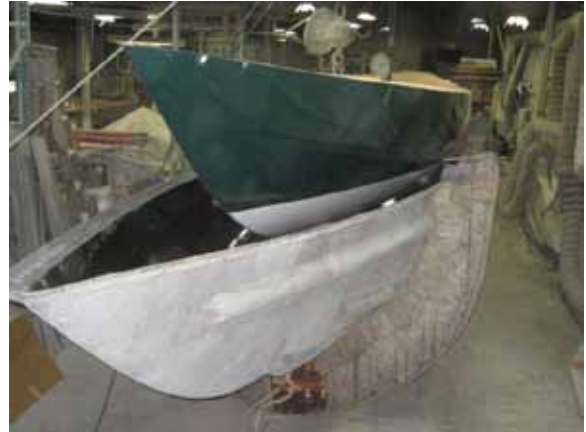
Removing the Boat from the Hull Mold
