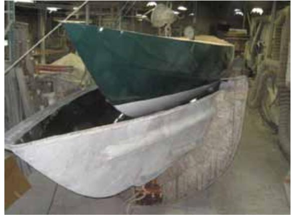
Removing the Boat from the Hull Mold
