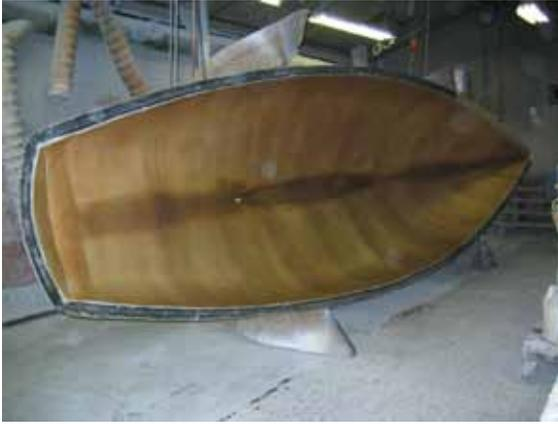
Shields Hull in Mold
