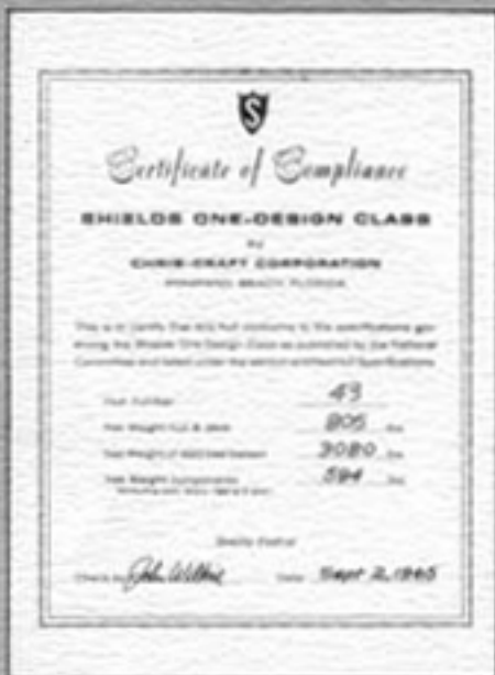
20. A replica of the Shields Certificate of Compliance, which every owner receives. Hull, deck, and components must be held within a 4% plus or minus weight, and the keel is 1% plus or minus the mean weight.
