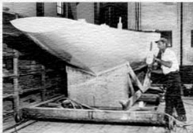
6. The topsides are buffed to a high luster. The color-impregnated hulls do not require painting. Hullside colors available are white, vermillion, light blue, dark blue, and green.
