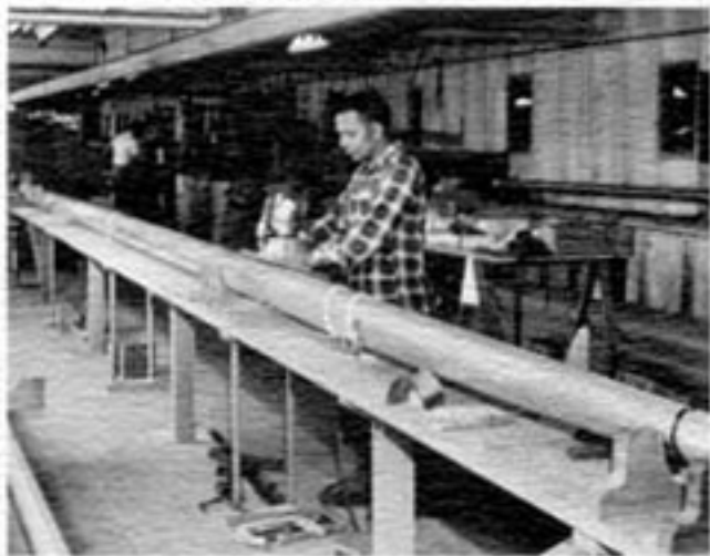
15. To assure uniformity in locating mast fittings, the masts are held in a jig while fittings are attached.
