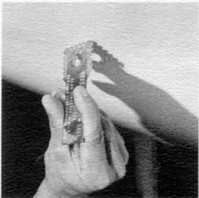
8. All gel coat applications are carefully checked for a thickness of .015". Gel coats that are too thick have a tendency to craze and check; if they're too thin, a scratch can remove all the color—or the color will not be opaque.
