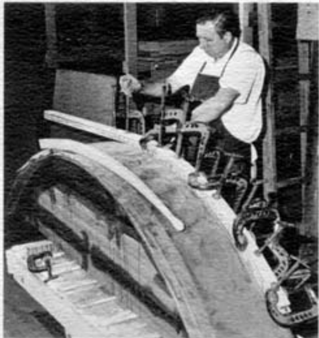
13. The white ash tiller is laminated in three pieces to maintain proper contour.
