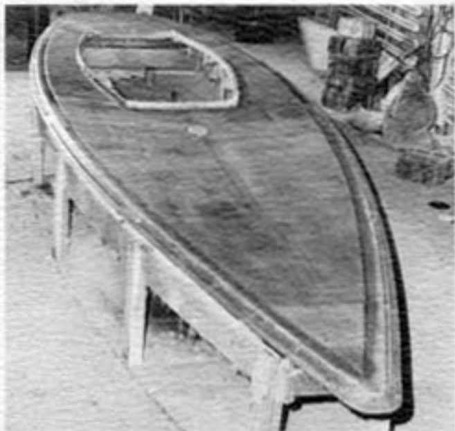
3. The one-piece deck is reinforced with plywood and overlaid with fiberglass.
