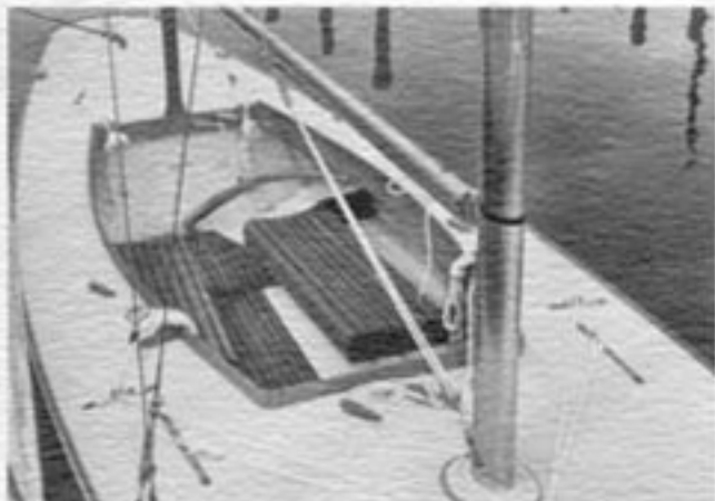
18. Deck and cockpit area. Hatches to compartments are watertight. Seats and trim are teakwood.
